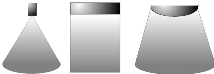
Shematski prikaz snopa talasa koje šalju u tkivo sektorska, linearna i konveksna sonda Schematic representation of the wave beams emitted into tissue by sector, linear, and convex probes.
